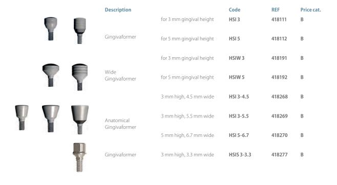
Screwable abutments for cemented bridges, without anti-rotation protection. Trimming and grinding is possible. Tighten with **HT 1.25**. Recommended insertion torque **20 Ncm**.
